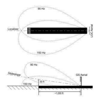
Normally approaching aircraft will be flying at an altitude which places them at an altitude between 3000 feet and 4000 feet to pick up the glide-slope. At times it is possible that due to temporary restrictions an aircraft may be coming in higher than normal in these cases the approach clearance needs to include the advise to the pilot that he can follow the glide or not to follow the glide as the case may be.
