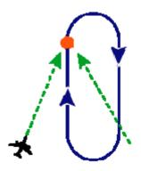
In a parallel entry, the aircraft flies to the holding fix, parallels the inbound course for one minute outbound, and then turns back, flies directly to the fix, and proceeds in the hold from there.
