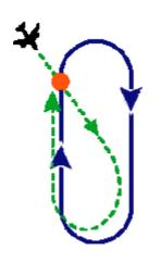
(b) The planned time along the inbound track is other than the standard one-minute or one-and-a-half minute leg appropriate for the altitude flown.
