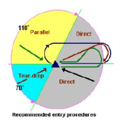
When crossing the fix to enter a holding pattern, the appropriate ATC unit shall be advised. ATC may also request that the pilot report "established in the hold". The pilot is to report "established" when crossing the fix after having completed the entry procedure.
