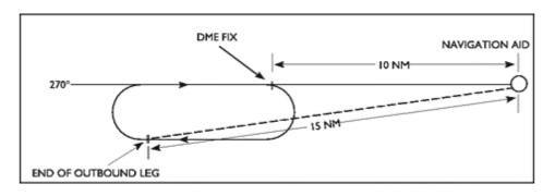
For example: An aircraft cleared to the 270° RADIAL 10 mile DME FIX, to HOLD BETWEEN 10 AND 15 miles, will hold inbound on the 270° radial, commence turn to the outbound leg when the DME indicates 10 NM and commence turn to inbound leg when the DME indicates 15 NM.
