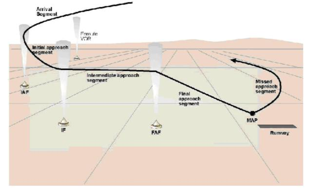
ATC may replace some or all (with the exception of the **FAF**) of these phases of the approach with radar vectors to the final approach, to allow traffic levels to be increased over those of which a fully procedural approach is capable. It is very common for ATC to vector aircraft to the final approach aid, e.g. the ILS, which is then used for the final approach. If traffic allows it or indeed if it becomes necessary then ATC can issue specific constraints on the approaching traffic:
